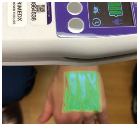
An AccuVein Vein Finder projects a map of a woman's veins for easy needle insertion at Sletten Cancer Institute.
